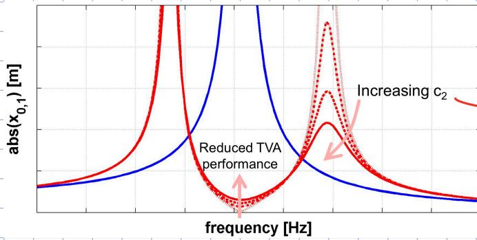
↑  $c_2$  reduces amplitude of new resonant frequencies but reduces performance of TVA in anti-resonance
